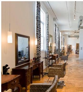
Evolution's old-fashioned and energy-intensive 90-watt halogen lamps failed annoyingly often and clashed with the salon's contemporary flair. The halogens were also expensive to operate and emitted so much heat that they increased air-conditioning costs in the summer. Swinney replaced 63 halogen PAR 38s in tracks throughout the reception area and studio floor with RVLT's dimmable 18-watt PAR 38s in warm white.
